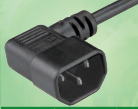
SL-30 (IEC 60320 C14) SVT 18AWG/3C SJT 18~14AWG/3C H05VV-F 0.75~1.0mm 2 /3G
