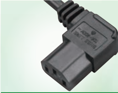
SL-11 (IEC 60320 C13) SVT 18AWG/3C SJT 18~14AWG/3C H05VV-F 0.75~1.5mm 2 /3G
