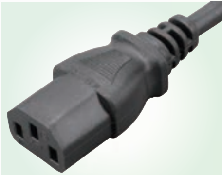
SL-3 (IEC 60320 C13) SVT 18AWG/3C SJT 18~14AWG/3C H05VV-F 0.75~1.5mm 2 /3G
