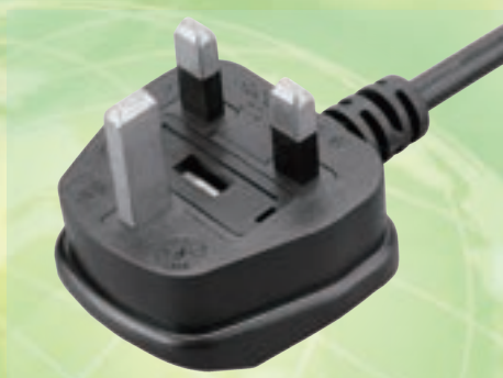
QP-026 (BS1363) H03VVH2-F, H05VVH2-F 0.75mm 2 /2C H03VV-F 0.75mm 2 /3G H05VV-F 0.75~1.5mm 2 /3G H05RN-F 0.75~1.0mm 2 /3G
