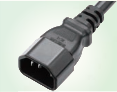
SL-4 (IEC 60320 C14) SVT 18AWG/3C SJT 18~14AWG/3C H05VV-F 0.75~1.5mm 2 /3G
